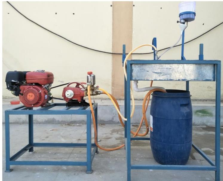
In this project we have designed and fabricated low-pressure abrasive water jet cutting head. Creo5.0 is used for drawings. Furthermore, project is fabricated as per design specifications. Our project is able to cut soft materials like rubber pad, bread bun, thermoplastic, sponge and soap. Additionally, gasoline engine of 6.5 hp is used as a power source for Triplex plunger pump.
